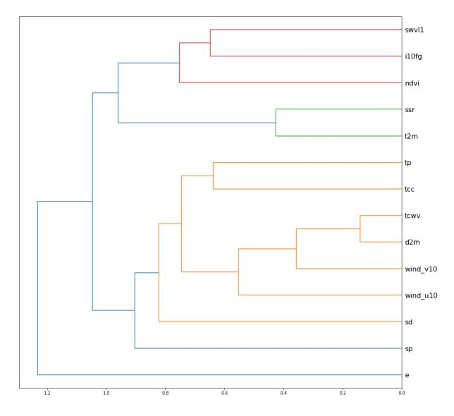
**Figure 4.** The above is a cross-correlation chart showing the relationships between features. Related features are connected by lines. The closer the line connecting the features is to the right-side of the graph, the more the features are related.
